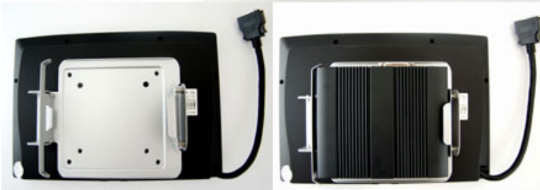
Example : QBOX mounted on CTF840-SH TFT display
